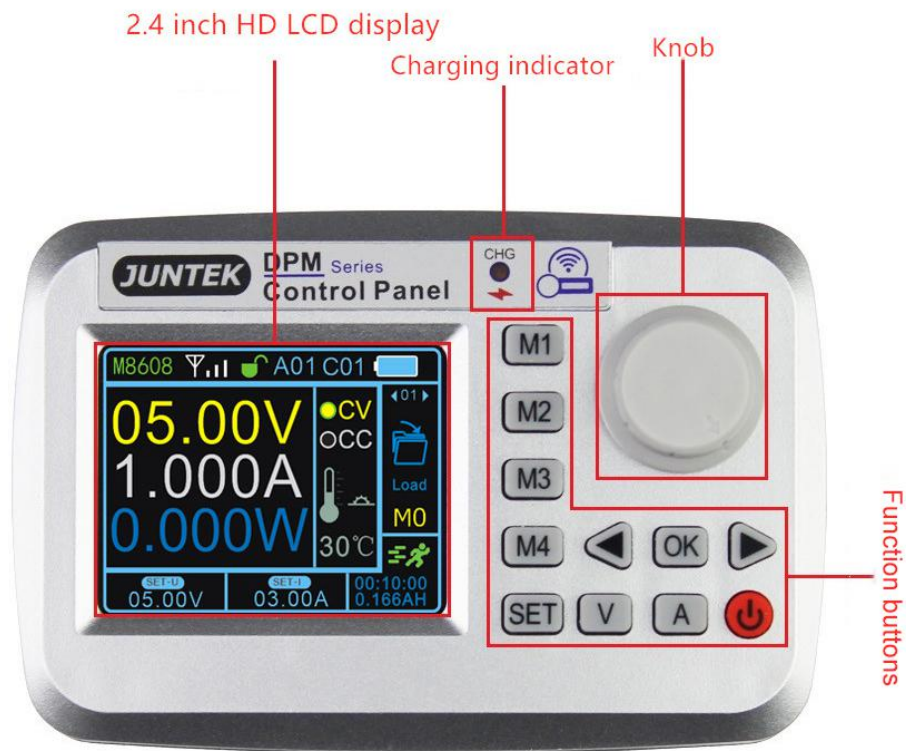
Figure 1-1 Wireless controller panel structure description
