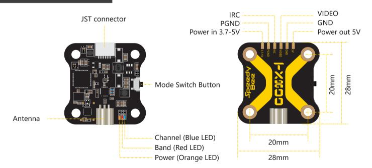
Notice: Please use the screws to install and fix the TX800 as the mainboard and the cover are separated.
