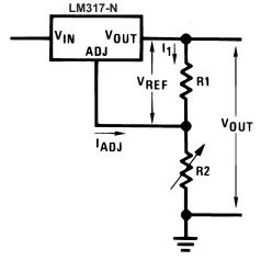
Figure 15. Setting the V<sub>OUT</sub> Voltage
