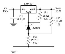
Figure 23. High Stability 10-V Regulator
