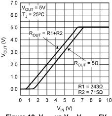
Figure 19.  $V_{OUT}$  vs  $V_{IN}$ ,  $V_{OUT}$  = 5V
