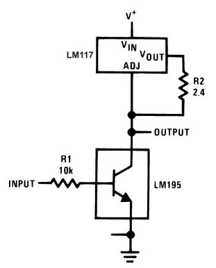
Figure 27. Common-Emitter Amplifier
