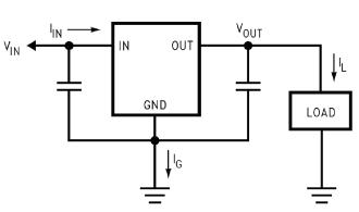
Figure 36. Power Dissipation Diagram
