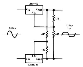
Figure 31. AC Voltage Regulator
