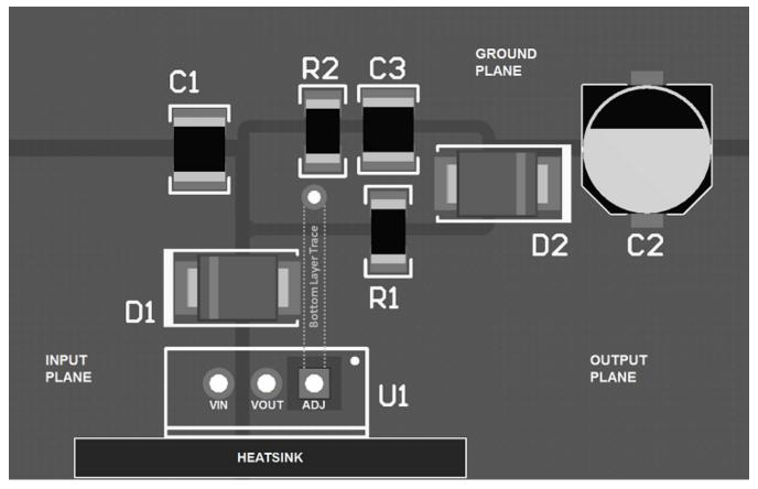
Figure 47. Layout Example (TO-220)
