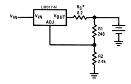
\*R<sub>S</sub>—sets output impedance of charger:  $Z_{OUT} = R_S \left(1 + \frac{R_2}{R_1}\right)$
