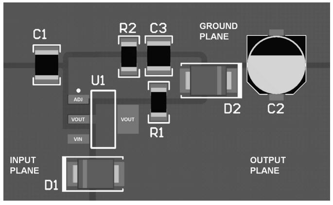
Figure 46. Layout Example (SOT-223)
