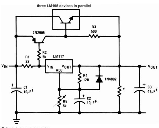
NOTE: ‡Optional—improves ripple rejection †Solid tantalum \*Minimum load current = 30 mA
