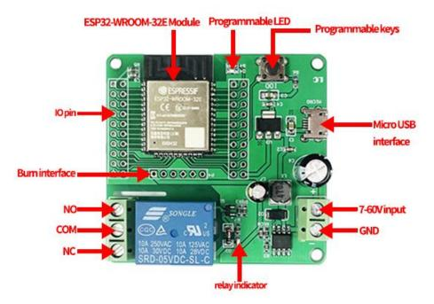
Programming port: GND, RX, TX, 5V of ESP32 are connected to GND, TX, RX, 5V of external TTL serial port module respectively. IO0 needs to be connected to GND when downloading, and then disconnect the connection between IO0 and GND after downloading;
