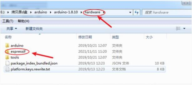
4, and then create a new blank folder named esp32 under the espressif folder
