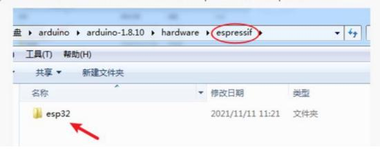
5. Unzip the downloaded compressed package and copy the content to the esp32 folder.
