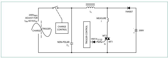
Note: Component values are for verification of rated (di/dt)c. See AN1048 for additional information
