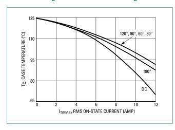
Figure 3. On-State Characteristics
